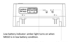
Running indicator: blue light turns on while MEGO is operating, or the device is being charged
